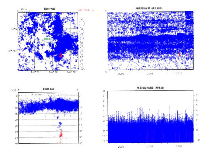
Figure 53-17 Activity of shallow VT earthquakes (blue circles) and deep low-frequency earthquakes (red circles) observed by a regional seismometer network (October 1, 1997, to June 30, 2012). Epicenter distribution (upper left), space-time plot (N-S cross-section) (upper right), E-W cross-section (lower left) and magnitude-time diagram (by scale) (lower right).
