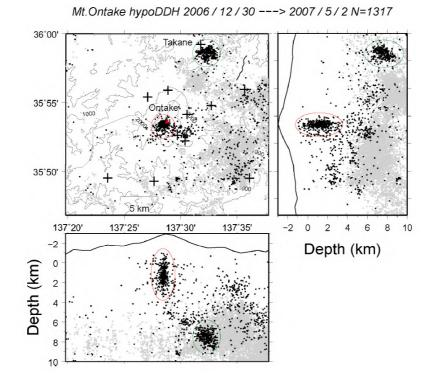
Figure 53-10 Distribution of earthquake hypocenters in and around the Ontakesan, determined by the Double Difference method (December 30, 2006, to May 2, 2007) (Nagoya University, 2007).
