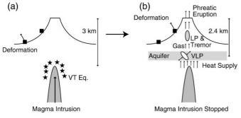
Figure 53-14 Very-long-period (VLP) earthquake mechanism in the 2007 phreatic explosion (Nakamichi et al, 2009).
