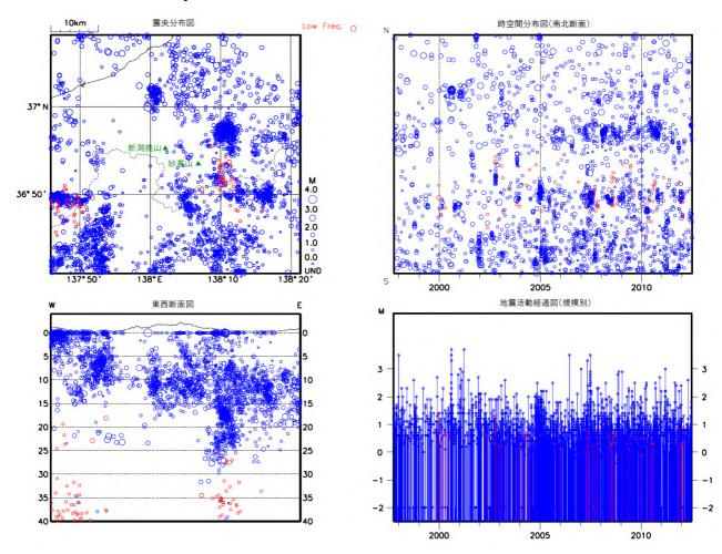
Figure 48-2 Activity of shallow VT earthquakes (blue circles) and deep low-frequency earthquakes (red circles) observed by a regional seismometer network (October 1, 1997, to June 30, 2012). Epicenter distribution (upper left), space-time plot (N-S cross-section) (upper right), E-W cross-section (lower left) and magnitude-time diagram (by scale) (lower right).
