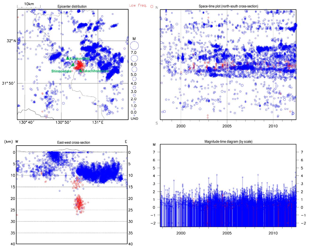
Figure 87-15 Activity of shallow VT earthquakes (blue circles) and deep low-frequency earthquakes (red circles) observed by a regional seismometer network (October 1, 1997, to June 30, 2012). Epicenter distribution (upper left), space-time plot (N-S cross-section) (upper right), E-W cross-section (lower left) and magnitude-time diagram (lower right).
