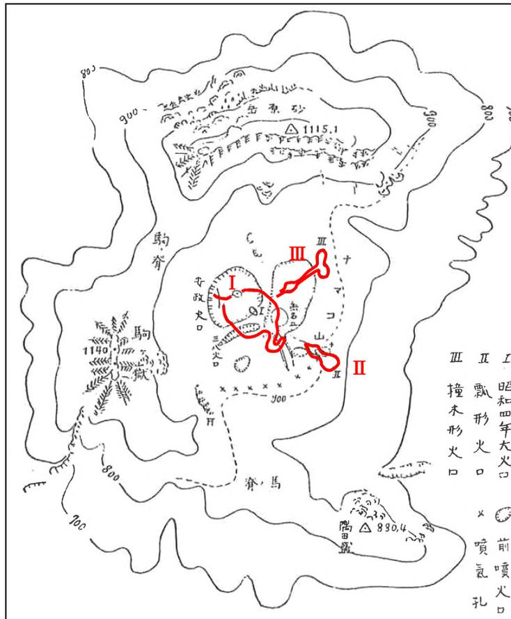
Figure 18-7 Changes in topography of Komagatake crater floor.
