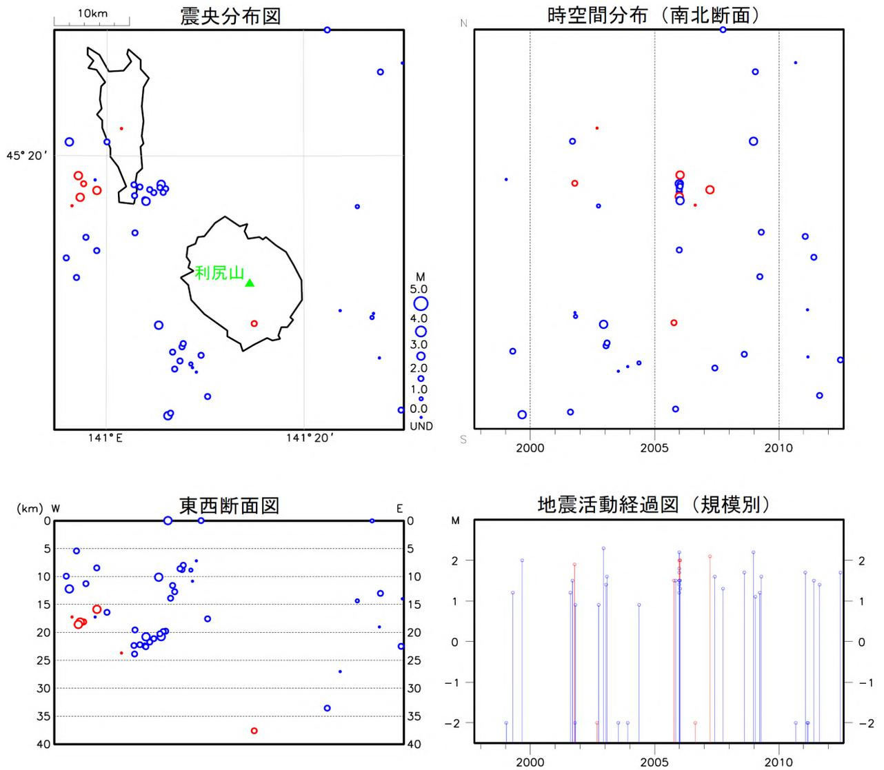
Figure 11-3 Activity of shallow VT earthquakes (blue circles) and deep low-frequency earthquakes (red circles) observed by a regional seismometer network (October 1, 1997, to June 30, 2012). Epicenter distribution (upper left), space-time plot (N-S cross-section) (upper right), E-W cross-section (lower left) and magnitude-time diagram (lower right).
