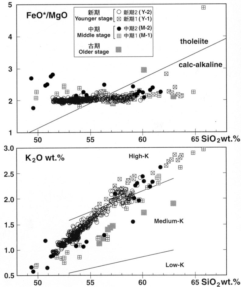
Figure 10-5 Whole rock chemical composition of Tokachidake volcano group by Harker diagram (Ishizuka et al., 2010).
