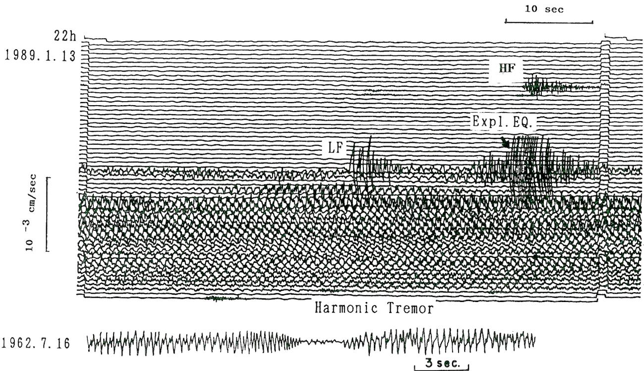
Figure 10-15 Records by short-period seismometer immediately before and after January 13, 1989 eruption (Okada et al., 1990).
