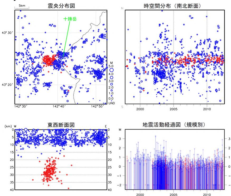
Figure 10-24 Activity of shallow VT earthquakes (blue circles) and deep low-frequency earthquakes (red circles) observed by a regional seismometer network (October 1, 1997, to June 30, 2012). Epicenter distribution (upper left), space-time plot (N-S cross-section) (upper right), E-W cross-section (lower left) and magnitude-time diagram (lower right).
