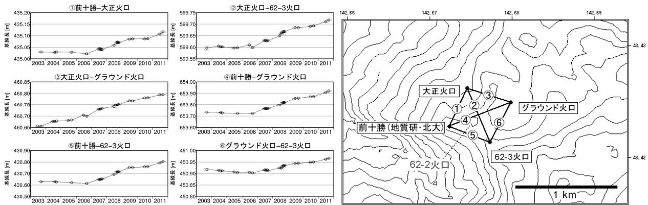
Figure 10-25 Crustal deformation in shallow area below 62-2 crater, observed by repeated GPS campaigns (2003 to 2011). (Japan Meteorological Agency, 2011)
