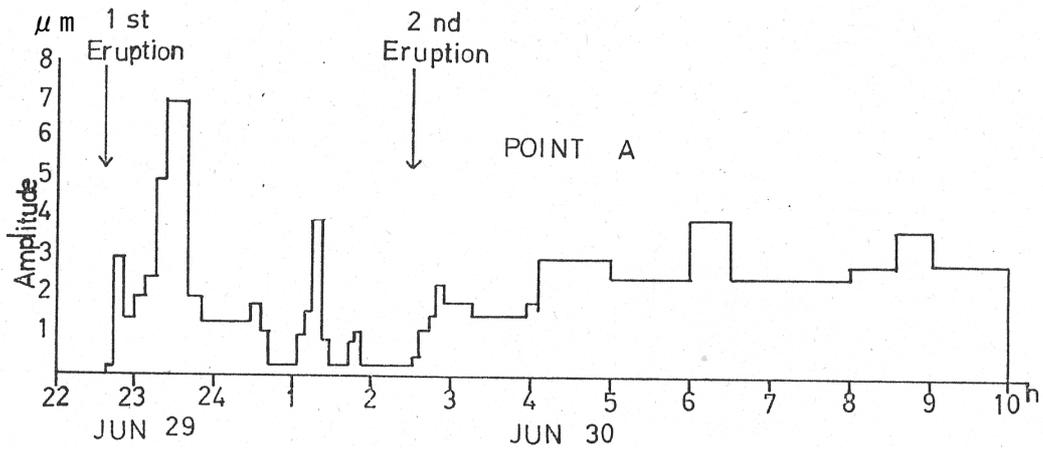
Figure 10-11 Changes in volcanic tremor amplitudes by the eruption on June 29 to June 30, 1962, measured at short-period seismometer (M-station, approximately 1.2km from crater) (Sapporo District Meteorological Observatory, 1971).
