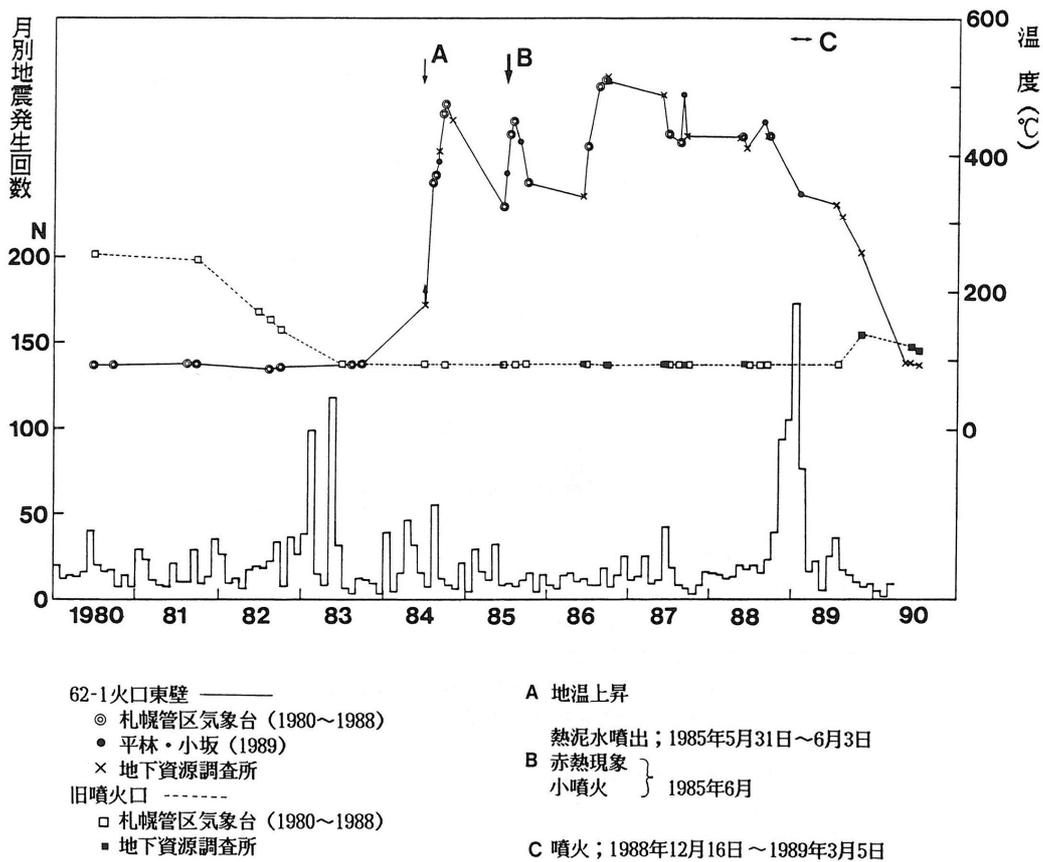
Figure 10-18 Changes in temperatures at 62-1 crater and old crater, and number of earthquakes per month (Akita et al., 1991).
