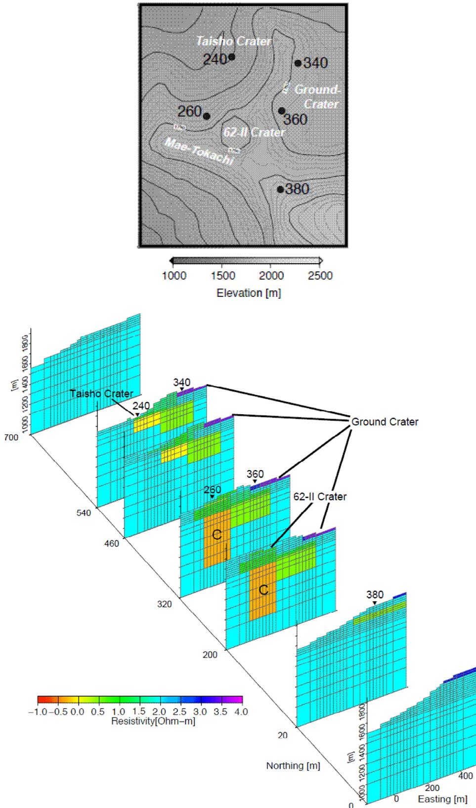
Figure 10-27 3D resistivity structure, determined via forward modeling (bottom) and observation point (top) (Yamaya et al., 2010).
