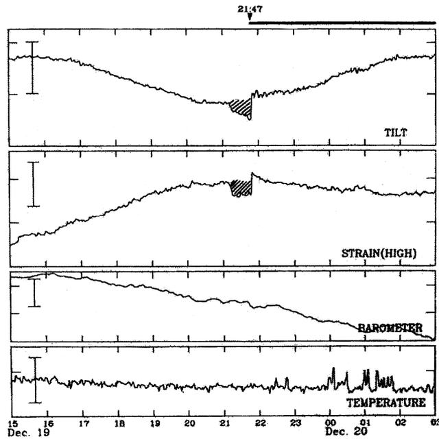
Figure 10-20 Changes in tiltmeter and strainmeter just before the eruption on December 19, 1988 (Miyamachi et al., 1990).
