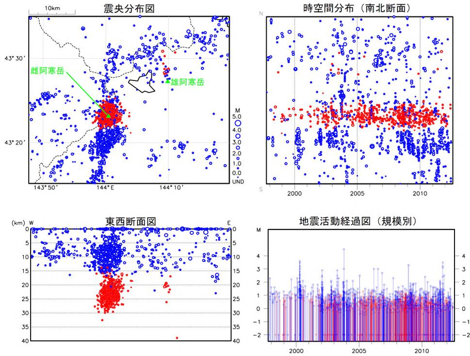
Figure 7-13 Activity of shallow VT earthquakes (blue circles) and deep low-frequency earthquakes (red circles) observed by a regional seismometer network (October 1, 1997, to June 30, 2012). Epicenter distribution (upper left), space-time plot (N-S cross-section) (upper right), E-W cross-section (lower left) and magnitude-time diagram (lower right).
