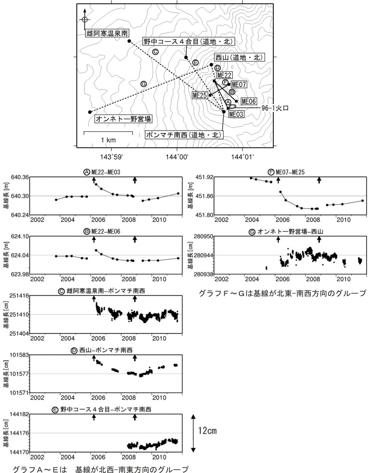
Figure 7-14 Changes of the GPS baselines (2003 to 2011, ↑ symbols represent eruptions) and observation points (Japan Meteorological Agency, 2011).
