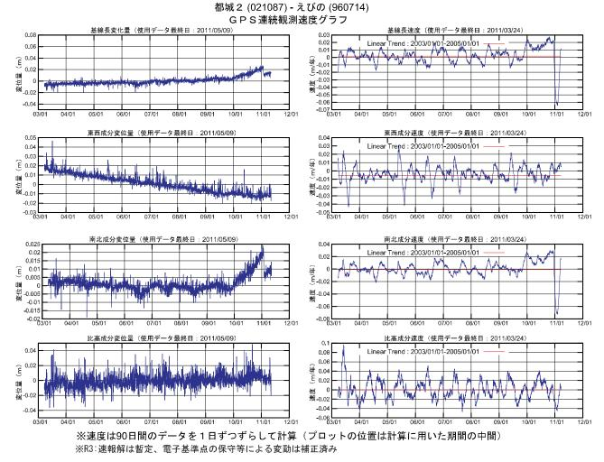
第4図(c) 霧島山周辺の GPS 連続観測結果(左列: 各成分時系列、右列: 各成分変化速度・90 日移動平均) Fig.4(c) Results of continuous GPS observation around Kirishima Volcano; (Left) Baseline length, E-W component, N-S component and Relative height, (Right) Time series of velocity for the baseline length by 90 days moving averages.
