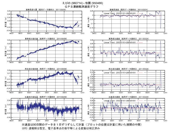
第4図(a) 霧島山周辺の GPS 連続観測結果(左列: 各成分時系列、右列: 各成分変化速度・90 日移動平均) Fig.4(a) Results of continuous GPS observation around Kirishima Volcano; (Left) Baseline length, E-W component, N-S component and Relative height, (Right) Time series of velocity for the baseline length by 90 days moving averages.
