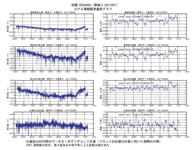
第4図(b) 霧島山周辺の GPS 連続観測結果(左列: 各成分時系列、右列: 各成分変化速度・90 日移動平均) Fig.4(b) Results of continuous GPS observation around Kirishima Volcano; (Left) Baseline length, E-W component, N-S component and Relative height, (Right) Time series of velocity for the baseline length by 90 days moving averages.
