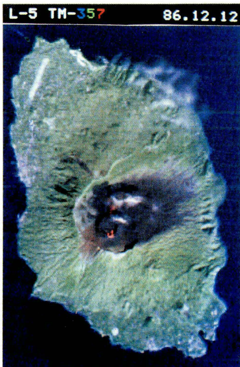
Fig.1 Detailed temperature of ground surface distribution on the southern part of Izu-Oshima Island on 12 December 1986 analysed from TM band 3, 5 and 7 data.
