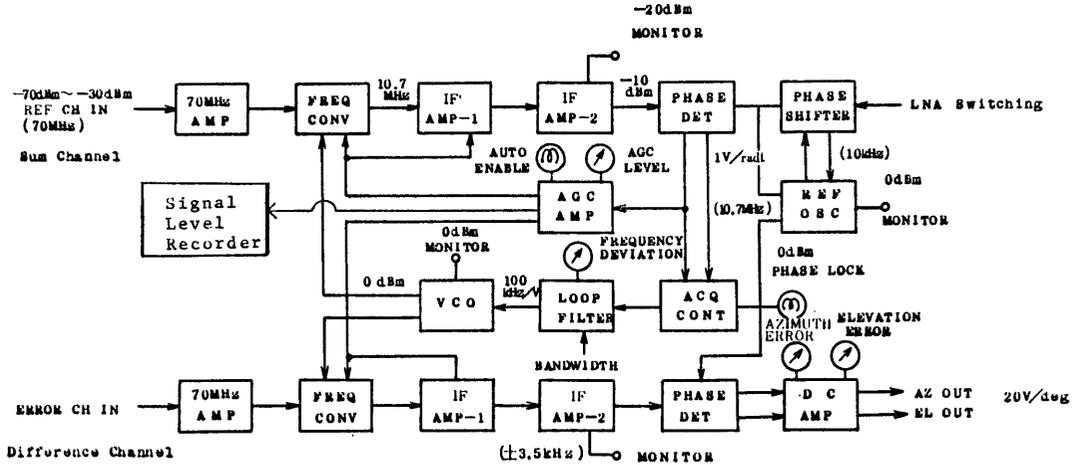
Fig. 5 Functional Block Diagram of the tracking receiver.
