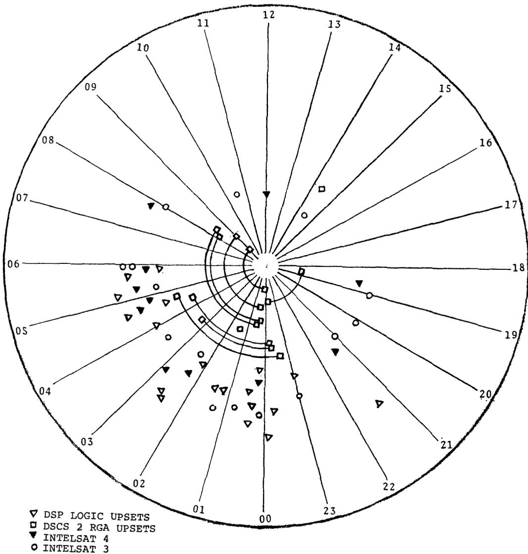
Fig. 9 Local time plot of various satellite disruptions and anomalies. The radial variations are not real but merely for graphical representation.
