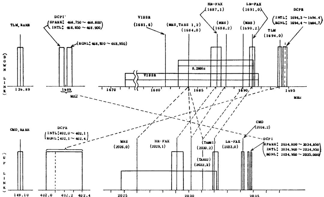
Fig. 3 Frequency allocation of the GMS up link and down link.
