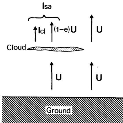
Fig.11 Sketch illustrating IR radiation from semitransparent cirrus. Upward flux of the long wave radiation from the ground is  $U$ , satellite observed radiation is  $I_{sa}$ , and the cloud radiation is  $I_{cl}$ .
