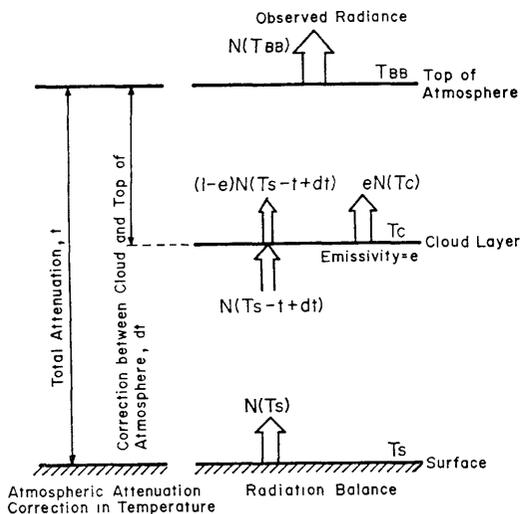
Fig. I-1 Schematic diagram of radiation balance in related to Eq. 1.
