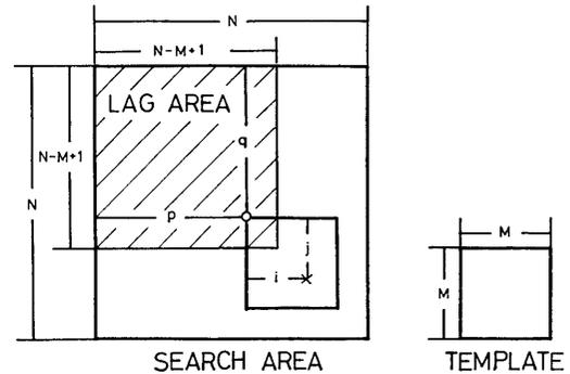
Fig. II-2 Schematic of search area and template area used for calculating cross-correlation matrix.
