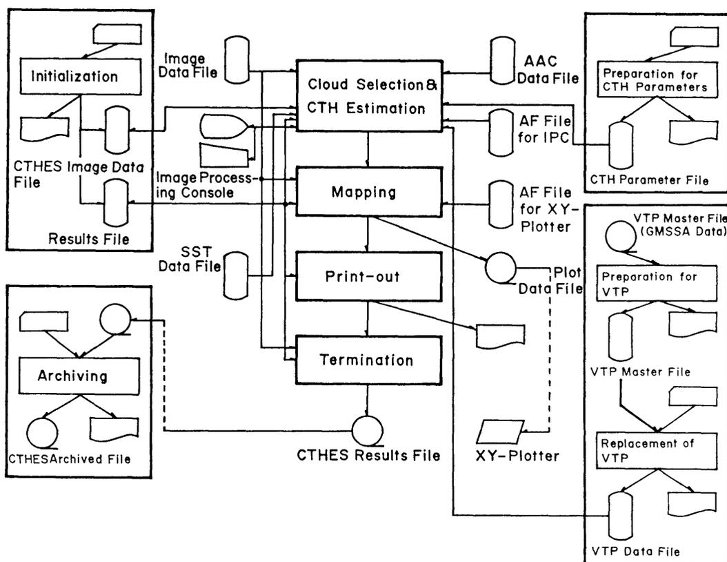
Fig. I-3 System configuration and functional block diagram of the CTHES.
