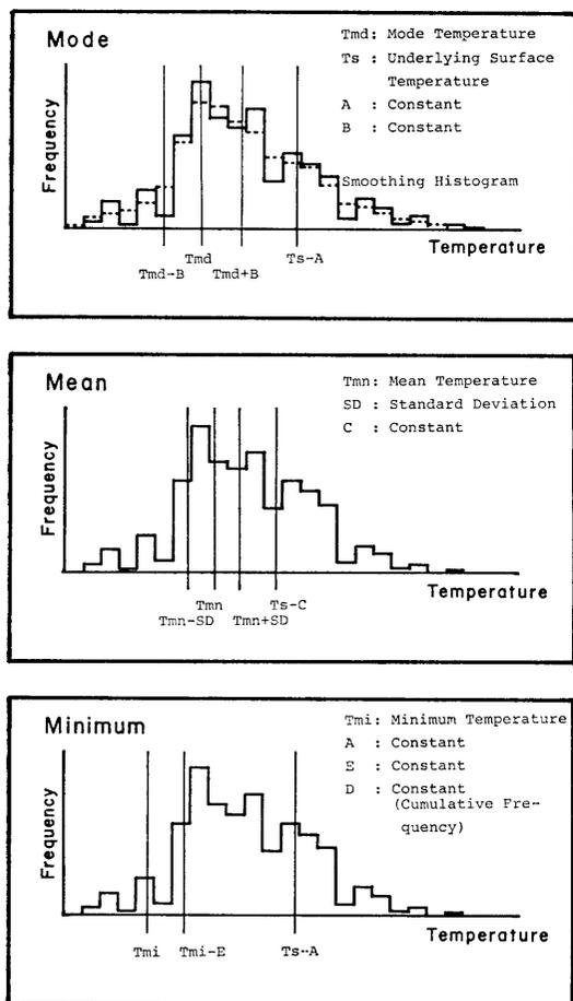
Fig. I-2 The diagram showing how to estimate representative temperature over target cloud area.
