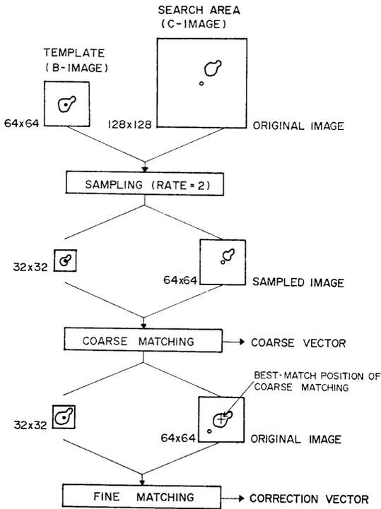
Fig. II-4 Schematic of double matching in CWES system. Sampling rate of coarse matching is given in the process of initial parameter set.
