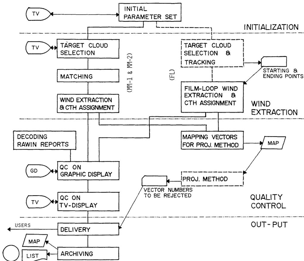
Fig. II-1 General flow of CWES system. "CTH" means cloud top height.
