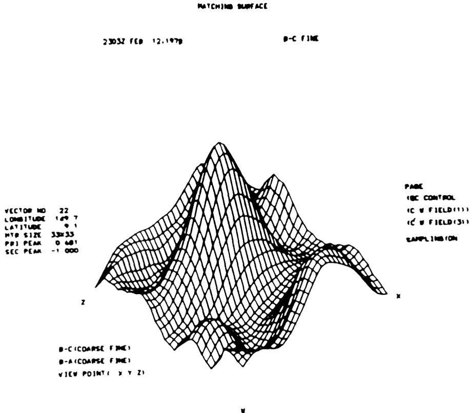
Fig. II-3 Matching surface displayed on the screen of a graphic display.
