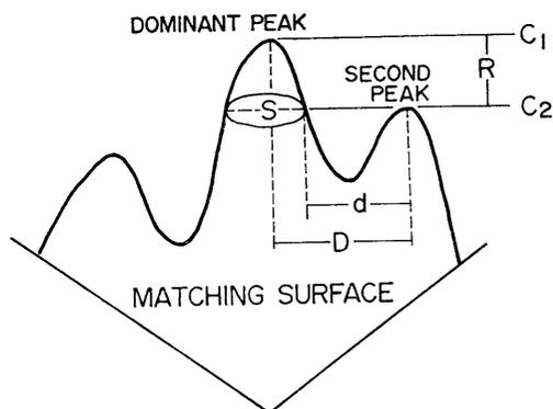
Fig. II-6 Parameterization of a matching surface with multiple peaks.
