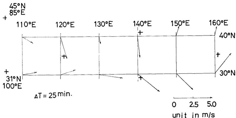
**Fig. 1** The distribution of error in magnitude due to poor registration. It is assumed that the information of satellite-attitude is good. The direction of arrows indicates the displacement of longitude/latitude intersection points. The plus mark “+” shows the position of bench mark by which error has been evaluated. Used imageries are taken at time from 0407Z to 0432Z.
