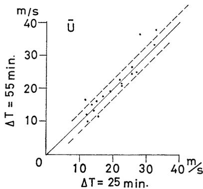
Fig. 4 The comparison of  $u$ -component in the time interval 25 minutes and 55 minutes. Broken lines indicate the range of error within  $\pm 2.2$  m/s.
