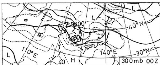
Fig. 12 The 300 mb chart at 0000Z June 27th 1978. The solid lines show contour, the interval of which is 120 meters. The dotted lines indicate iso-tach, the interval of which is 20 m/s. The area of more than 40 m/s in wind speed is stippled.
