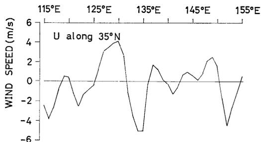
Fig. 9 Smaller scale waves on a  $u$ -field extracted from interpolated data by the running mean method. The ordinate corresponds to a scale of an amplitude of the wave, the abscissa corresponds to a scale of a wave length, respectively.
