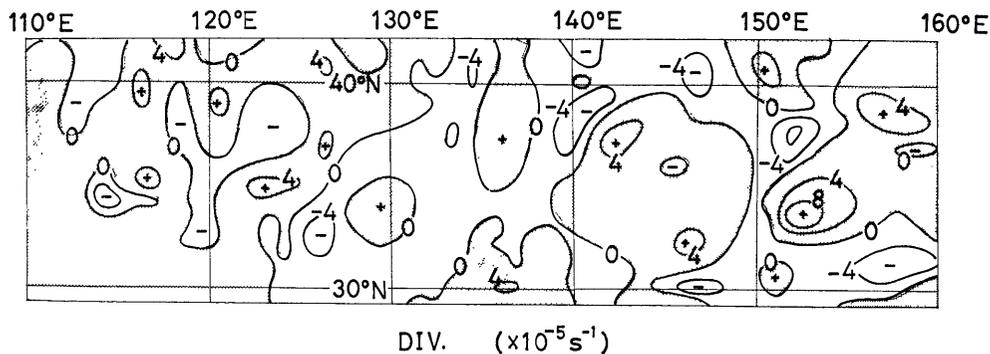
Fig. 13 The divergence field calculated from interpolated  $u$ - and  $v$ -component, in which  $1^\circ$  longitude/latitude is used as the grid interval. Positive areas are stippled. Unit is in  $\times 10^{-5} \text{ sec}^{-1}$  and interval of iso-value is 4.
