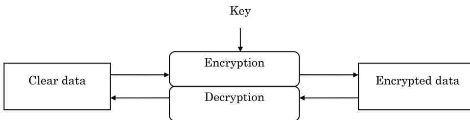
**Figure 5-9** Encryption Principle
