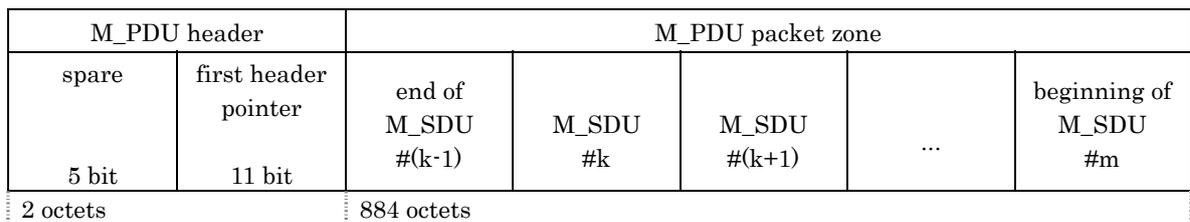
**Figure 8-1 M\_PDU Structure**
