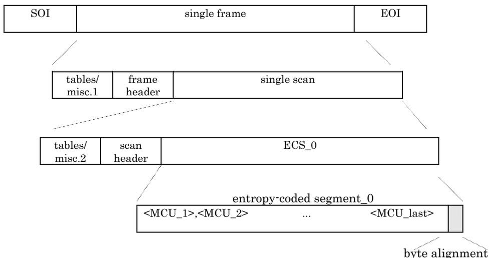
**Figure 5-4 JPEG structure of compressed image data**
