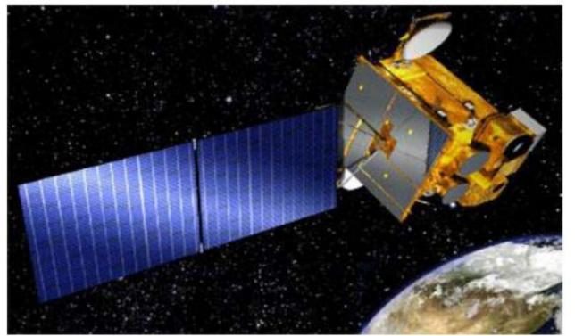
COMS (Chollian), the first Korean multi-function geostationary satellite (Communication, Ocean and Meteorological Satellite). Launched on 27/6/2010, Operational at 138° East. Wavelength : VIS,IR1,IR2,watervapor, NIR Spatial resolution : 1km × 1km, 4 km×4km Temporal resolution : 15min
