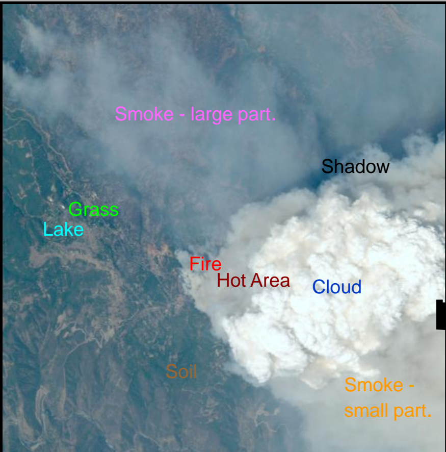
AVIRIS Image - Linden CA 20-Aug-1992 224 Spectral Bands: 0.4 - 2.5 \mu\text{m} Pixel: 20m x 20m Scene: 10km x 10km
