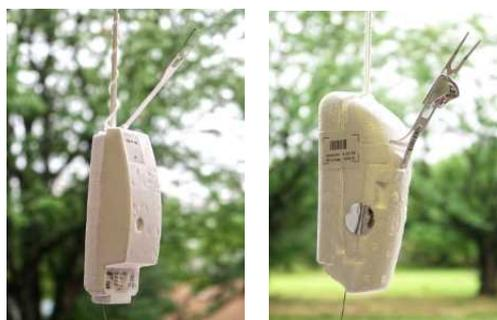
Photo 1 Model RS41 (left) and iMS (right) GPS sondes.
