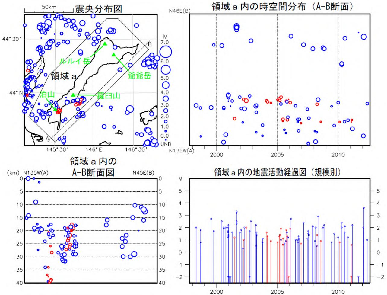
Figure 107-2 Activity of shallow VT earthquakes (blue circles) and deep low-frequency earthquakes (red circles) observed by a regional seismometer network (October 1, 1997, to June 30, 2012). Epicenter distribution (upper left), space-time plot (A-B cross-section) of "a" region (upper right), A-B cross-section of "a" region (lower left) and magnitude-time diagram of "a" region (lower right).
