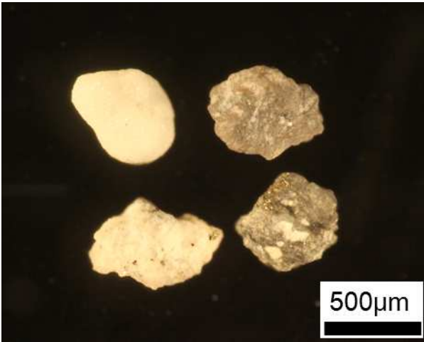
第4図 白色・灰色岩片の实体顕微鏡写真 Fig.4 Photomicrograph of white and gray lithic fragments in washed volcanic materials emitted from the site of the geothermal power plant in Ioto Island on December 16, 2014.
