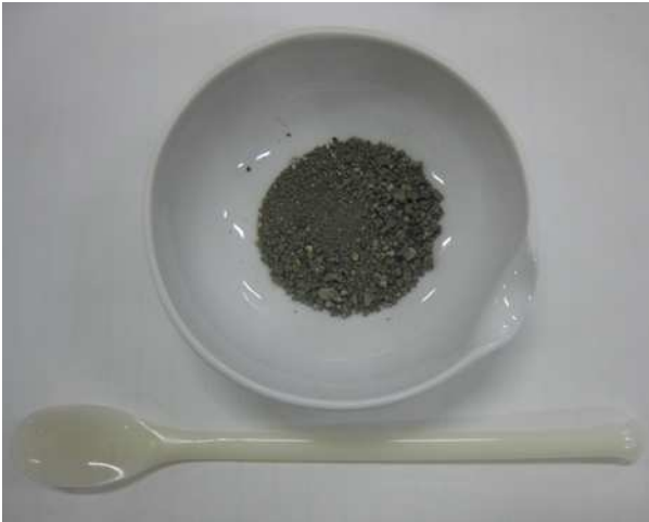
第1図 水洗前の噴出物の写真 Fig.1 Photograph of unwashed volcanic materials emitted from the site of the geothermal power plant in Ioto Island on December 16, 2014.
