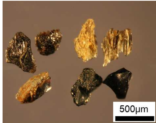
第 9 図 火山ガラス片の実体顕微鏡写真 Fig.9 Photomicrograph of volcanic glass fragments in washed volcanic materials emitted from the site of the geothermal power plant in Ioto Island on December 16, 2014.
