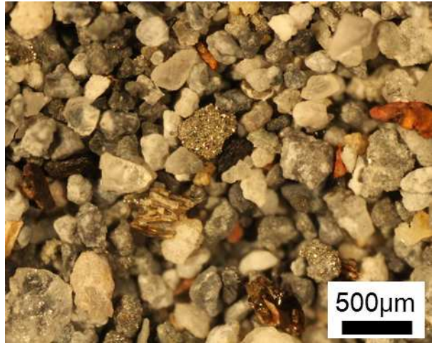
第2図 水洗後の噴出物(粒径250µm - 500µm残渣粒子)の実体顕微鏡写真 Fig.2 Photomicrograph of washed volcanic materials (grain size: 250µm-500µm) emitted from the site of the geothermal power plant in Ioto Island on December 16, 2014.
