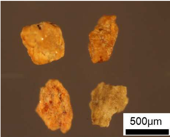
第 8 図 硫酸塩鉱物集合体の実体顕微鏡写真 Fig.8 Photomicrograph of sulfate mineral aggregates in washed volcanic materials emitted from the site of the geothermal power plant in Ioto Island on December 16, 2014.
