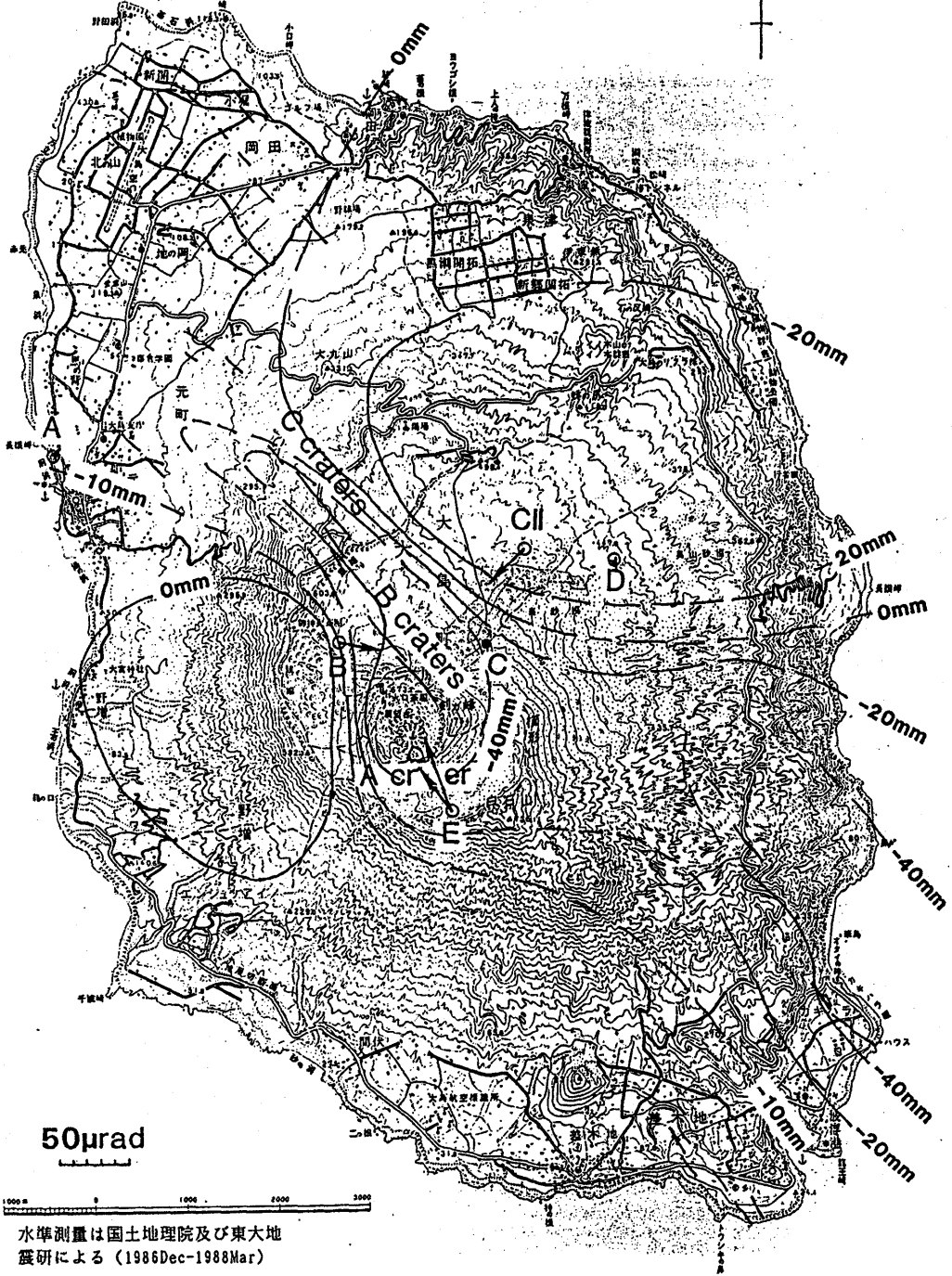
第1図 各観測網における最大傾斜 (Down tilting) の方向 Fig.1 Localities of survey nets and azimuths of down-tilting during May 1989 and Sep. 1989.
