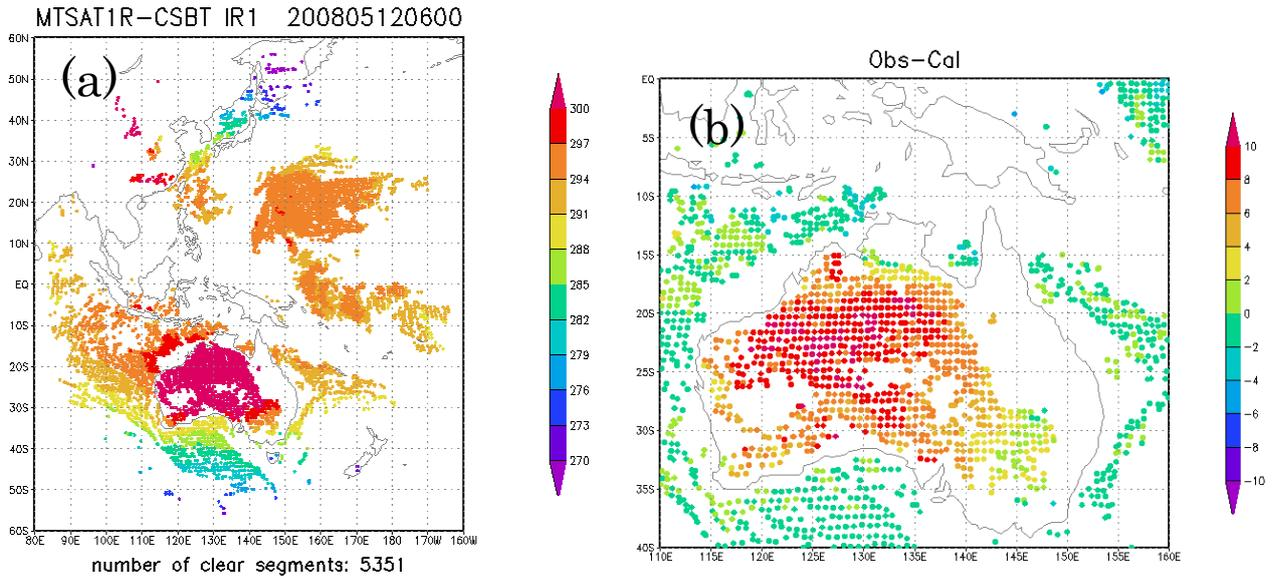
**Figure 4. A comparison of the MTSAT-1R window channel (IR10.8) CSR [as TB (K)] with the expected TBs (K) calculated from the JMA global model 6-hour forecast first-guess fields using RTTOV-9 for 06 UTC May 12, 2008: (a) MTSAT-1R IR10.8 CSR data; (b) Difference of MTSAT-1R IR10.8 CSR minus first-guess values for the Australian region (110°E–160°E and 0°S–40°S). Neither bias correction nor quality controls are applied.**
