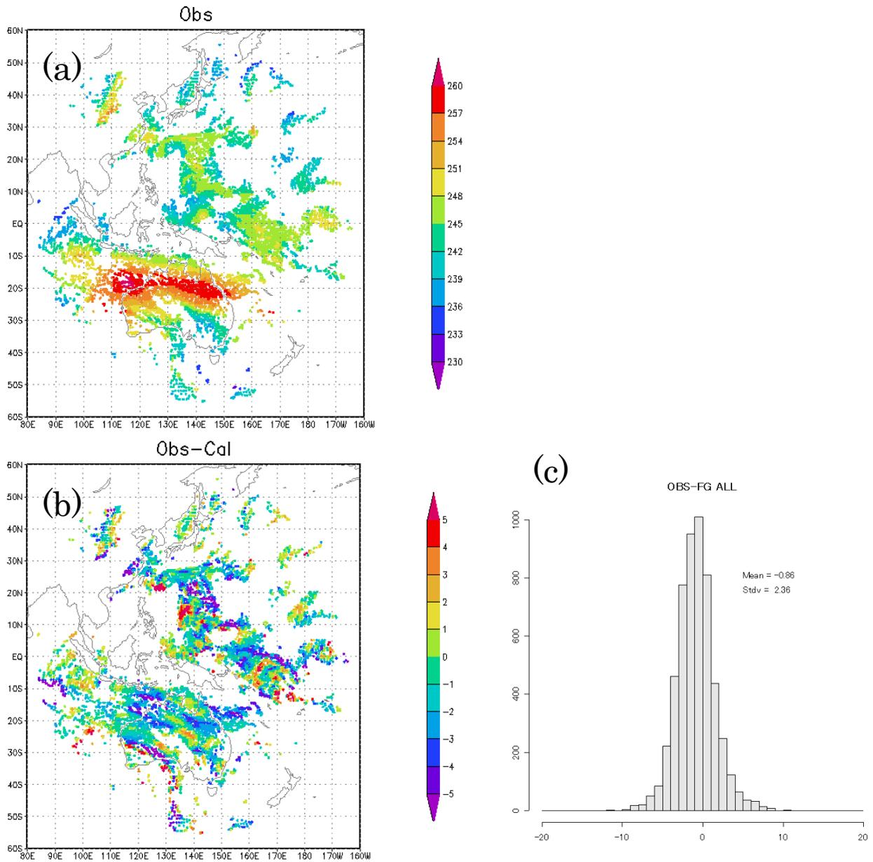
**Figure 3. A comparison of the MTSAT-1R water vapor (WV) CSR [as TB (K)] with the expected TBs (K) calculated from the JMA global model 6-hour forecast first-guess fields using RTTOV-9 for 12 UTC July 5, 2008: (a) MTSAT-1R WV CSR data; (b) Difference of MTSAT-1R WV CSR minus first-guess values; (c) Histogram for departures of TB (K) between the CSR and model first guess. Neither bias correction nor quality controls are applied.**
