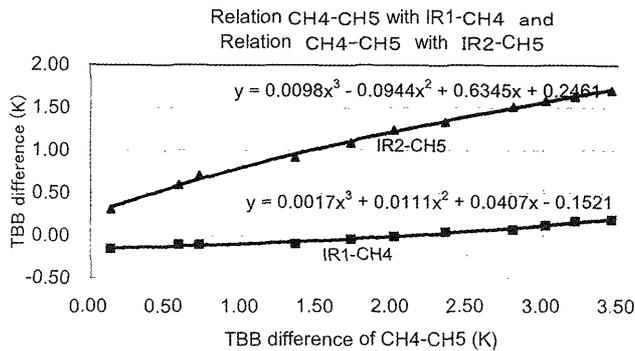
Fig. 3 Relation between the approximation formula and the result of the calculation by LOWTRAN7.
