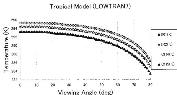
Fig. 1 Brightness temperature theoretically measured by GMS-5 and NOAA-16 for a tropical standard atmosphere (a value of sea surface temperature is 300 K) as a function of satellite viewing angle.
