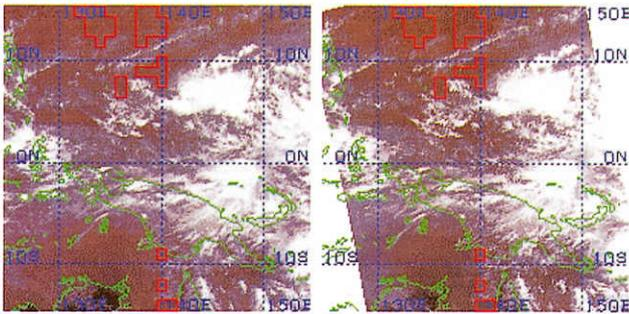
Fig. 2 A sample figure after passing information about space and time conditions and viewing geometry conditions, and removing cloud conditions. The left hand figure is from GMS-5, and the right hand is NOAA-16. Boxed areas show target areas.
