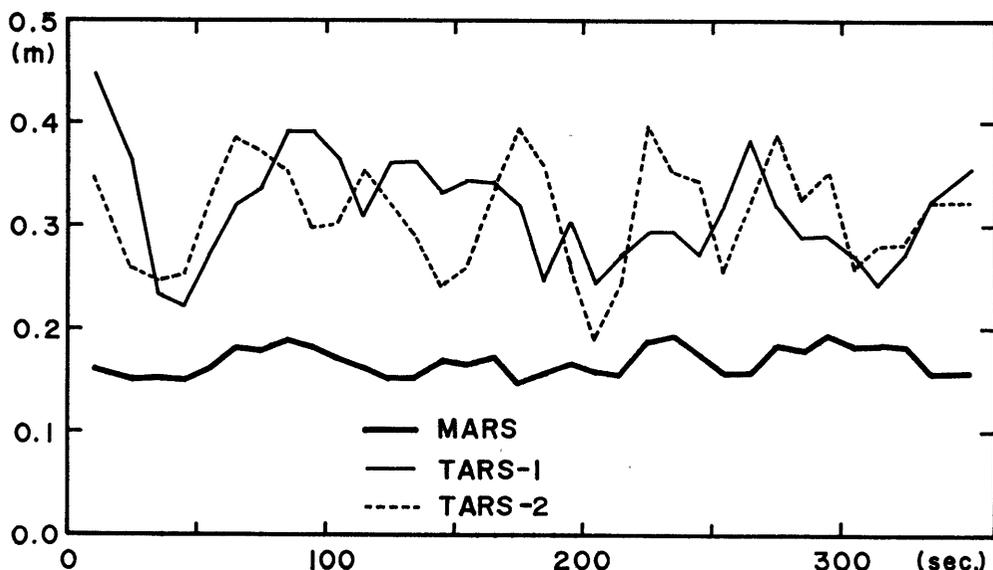
Fig. 3 An example of the temporal variations of the random errors of the ranging data. The numbers on the abscissa mean the time from the start of the ranging in seconds, and the numbers on the ordinate mean the magnitude of the random errors which are the standard deviations in meters around the least square approximations expressed with Chebyshev polynomials of the third order.
