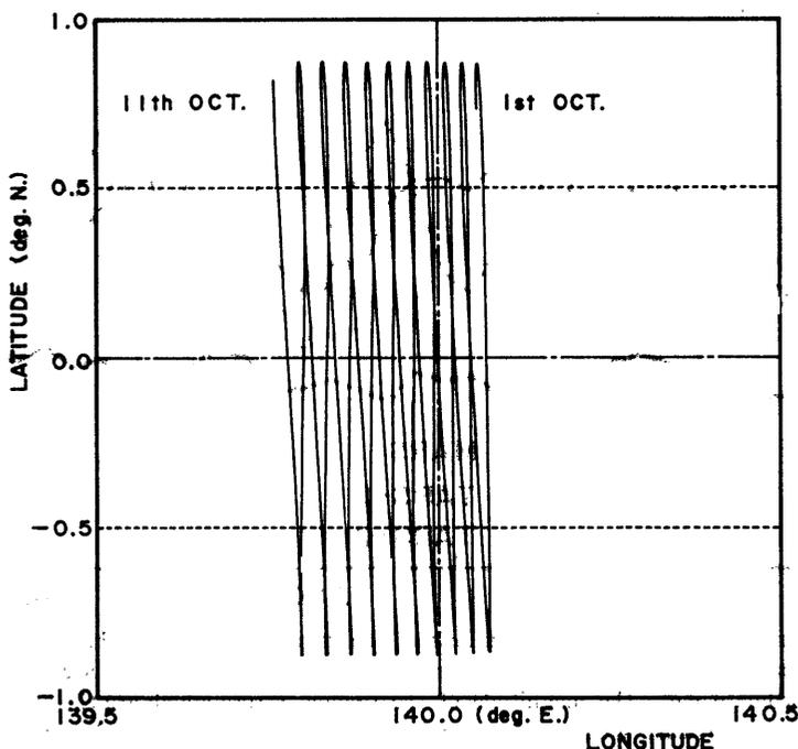
Fig. 2 An example of the temporal variations of the subsatellite point of GMS from 00: 00 UT, 1 Oct to 24: 00 UT, 11 Oct, 1980.
