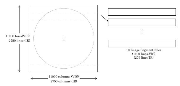
Figure A-1 Segmentation of full Earth's disk
