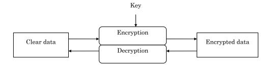
Figure 5-9 Encryption Principle
