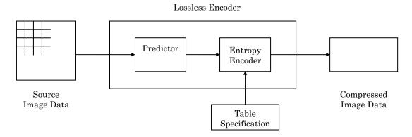
Figure 5-3 JPEG Lossless Image Compression Scheme
