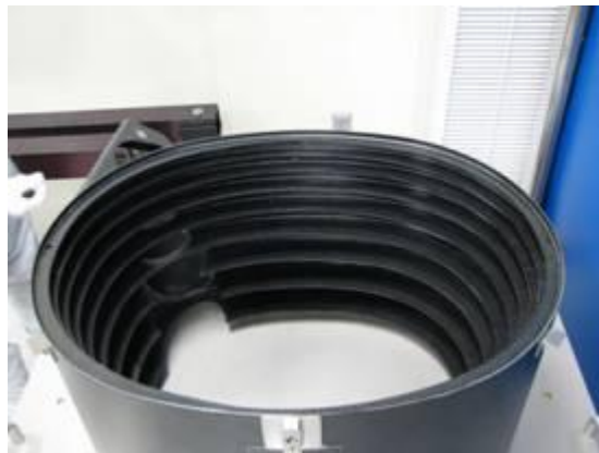
Optical Port Sunshield Assembly Stray Light Baffles
